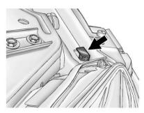
12. Push down on the plastic headlamp retainer to reinstall it.
